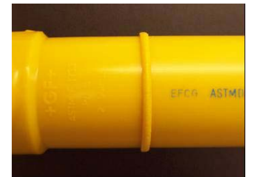
Examples of Acceptable Fusions of PA-11 Pipe to PA-11 Fitting
