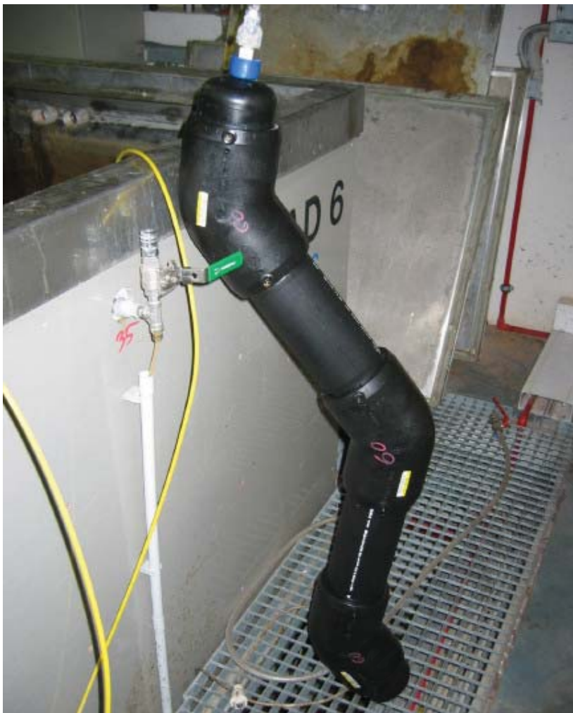
Photo 4: Internal (burst) pressure test at a testing stand in accordance with FM standard 1610
